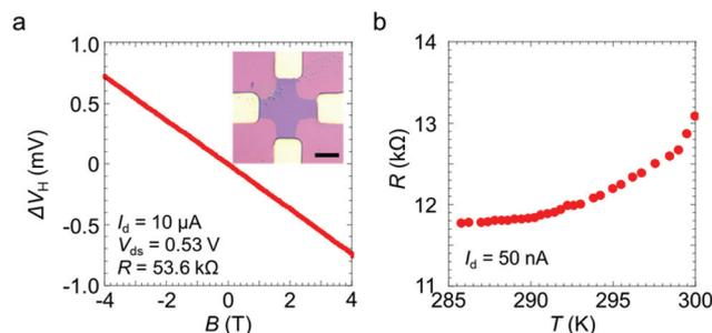
Fig. 2 (a) Magnetic field dependence of the Hall voltage for the doped monolayer  $\text{MoS}_2$  using  $100$  mM dopant solution at room temperature. The inset is an optical image of the sample. The scale bar is  $10 \mu\text{m}$ . (b) Temperature dependence of the electrical resistance for the doped monolayer  $\text{MoS}_2$  using  $100$  mM dopant solution.
