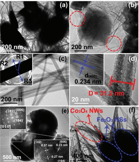
Fig. 2 TEM images of  $rGO/Co_3O_4@Fe_2O_3$  hybrid networks. (a) and (b) TEM results of the  $rGO/Co_3O_4@Fe_2O_3$  hybrid networks. (c) and (d) TEM results of  $Co_3O_4$  NWs. The insets in (c) and (d) show the SAED for the  $Co_3O_4$  NWs and the HRTEM image for the  $Co_3O_4$  NW region. (e) TEM results for  $Fe_2O_3$  NSs. The inset in (e) shows the SAED for the  $Fe_2O_3$  NS region. (f) TEM results of the  $Fe_2O_3$  NS interconnected region in the hybrid networks.
