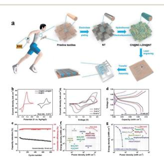
**Fig. 2** (a) Fabrication process of Co–Zn alkaline microbattery. (b) Cyclic voltammetry curves of CH@NC-LDH@NT and Zn@CC at 5 mV s $^{-1}$ . (c) Cyclic voltammetry curves, (d) galvanostatic charge/discharge curves, (e) long-term cycling stability, and (f and g) Ragone plots of Co–Zn alkaline MB. Reproduced with permission. <sup>27</sup> Copyright 2020, Wiley-VCH.
