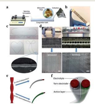
Fig. 7 (a) Schematic illustration of sinning process of the MXene/PU fiber. (b) Digital photograph of fabricated MXene/PU fiber. Reproduced with permission. Copyright 2020, Wiley-VCH. (c) Flexibility demonstration and SEM image of the yarn. (d) Demonstration of weavability and knittability. (e) Schematics of yarns electrodeposited with Zn and NCHO and (f) solid-state yarn battery. Reproduced with permission. Copyright 2017, American Chemical Society.
