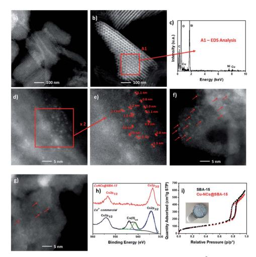
Fig. 2 (a and b) HAADF-HRSTEM analysis of Cu-NCs@SBA-15 with the selection of an area of 4  $\mu$ m<sup>2</sup> and (c) its relative EDS analysis. (d-g) HAADF-HRSTEM analysis of Cu-NCs smaller than 2 nm. (h) Cu 2p XPS core level of Cu-NCs@SBA-15 in red and Cu(ii) pattern in black showing the characteristic satellite peaks. (i) N<sub>2</sub> adsorption curve for the mesoporous substrate and the Cu-NC@SBA-15 catalyst.
