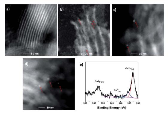
Fig. 3 (a-d) HAADF-HRSTEM analysis and (e) Cu 2p XPS spectrum of the heterogeneous catalyst after 3<sup>rd</sup> cycle at 100 °C for 20 h in 1,4-dioxane.
