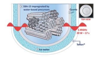
Fig. 1 Schematic representation and optical inset of the coaxial reactor for the simultaneous cooling–microwave heating.
