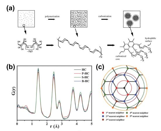
Fig. 14 (a) Hydrothermal reaction mechanism of hard carbon synthesis. <sup>96</sup> Copyright 2004, Wiley. (b) PDF profiles of heteroatom-doped hard carbon samples and (c) schematic illustration of local structure of graphene to help understand Fig. 14b. <sup>83</sup> Copyright 2017, Wiley.
