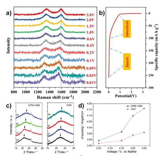
Fig. 7 In situ Raman spectra (a) with corresponding discharge states (b).<sup>47</sup> Copyright 2021, Elsevier. XRD profiles (c) with corresponding *d*-spacing of (002) crystal plane(d).<sup>48</sup> Copyright 2013, American Chemical Society.
