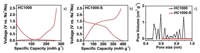
Fig. 8 GCD curves of HC samples without (a) and with sulphur filling in pores (b). (c) DFT pore size distribution curves of samples before (HC1000) and after sulphur filling (HC1000-S).<sup>52</sup> Copyright 2018, Wiley.
