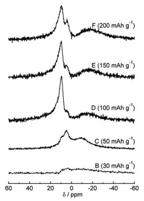
Fig. 11  $\,^{23}$ Na MAS NMR spectra at various states of charge.  $^{53}$  Copyright 2013, Elsevier.
