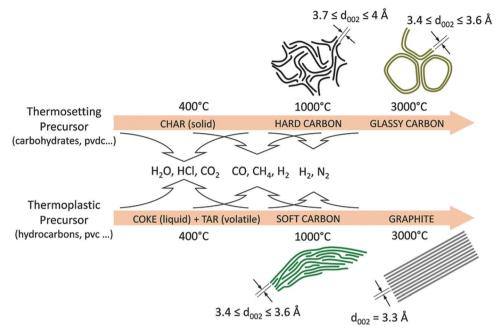
Fig. 3 Schematic illustration of the evolution of the microstructures of graphite, soft and HCs from different biomass precursors as a function of thermal treatment temperatures. <sup>36</sup> Copyright 2018, Wiley.
