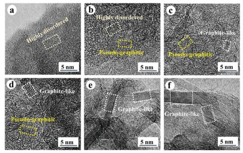
Fig. 25 High resolution transmission electron microscopy (HRTEM) images of HC samples pyrolysed at (a) 600, (b) 1000, (c) 1300, (d) 1700, (e) 2000 and (f) 2500  $^{\circ}$ C. Copyright 2019, Wiley.
