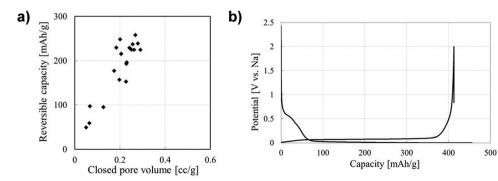
Fig. 24 (a) Correlation between closed pore volume and reversible capacity of sucrose derived HC. (b) GCD profile for sucrose derived HC. 157 Copyright 2015, IOPscience
