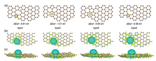
Fig. 21 Computational simulations of sodium-ion adsorbed on di-vacancy defects of Types 1–3 and single-vacancy defects of Type 4 in HC viewed from top (a and b) and side (c).<sup>82</sup> Copyright 2020, Wiley.
