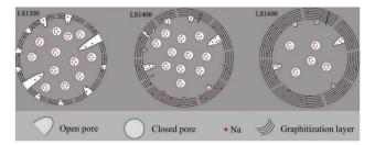
Fig. 16 Illustration of the evolution of porosity as a result of increasing thermal treatment at 1200  $^{\circ}$ C (LS1200), 1400  $^{\circ}$ C (LS1400) and 1600  $^{\circ}$ C (LS1600).  $^{58}$  Copyright 2018, Elsevier.
