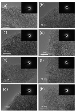
Fig. 19 TEM images showing the crystallite size of sucrose-derived HC samples pyrolysed at (a) 700, (b) 900, (c) 1100, (d) 1300, (e) 1500, (f) 1600, (g) 1800, and (h) 2000 °C.84 Copyright 2020, American Chemical Society.
