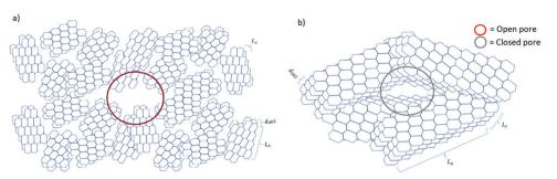
Fig. 15 Schematic comparison of the microstructural features of HC materials prepared at (a) low and (b) high pyrolysis temperatures.
