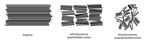
Fig. 2 Scheme illustrating the microstructures of graphite, soft carbon and hard carbon.<sup>34</sup> Copyright 2001, Wiley.
