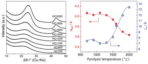
Fig. 18 (a) XRD patterns of sucrose-derived HC samples pyrolysed at temperatures between 700 and 2000 °C, and (b) relationship between d-spacing and graphitic crystallite length along the c-axis as a function of pyrolysis temperature.<sup>84</sup> Copyright 2020, American Chemical Society.
