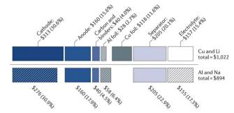
Fig. 1 A cost comparison between lithium-ion and sodium-ior batteries. <sup>13</sup> Copyright 2001, Springer Nature.
