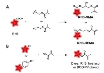
Fig. 13 Transformation of fluorophores into dye-methacrylate monomers by esterification with GMA or HEMA (A) or by esterification of methacryloyl chloride (B).
