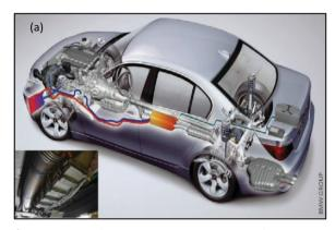
Fig. 18 Integration of thermoelectrics into vehicles for improved fuel efficiency. The image is a BMW 530i concept car with a thermoelectric generator (yellow; and inset) and radiator (red/blue). Reprinted by permission from (Springer Nature), (Nat. Mater.) ref. 182 (An inconvenient truth about thermoelectrics, C. B. Vining, 8 (2009) 83-85), Copyright 2009.
