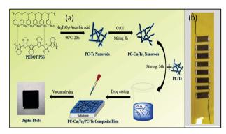
Fig. 14 (a) Schematic of the steps for the fabrication of PC-Cu7Te4/ PC-Te composite film and (b) photograph of a fabricated TE device by using as-prepared film. Reprinted with permission from ref. 159 (Y. Lu, Y. Qiu, Q. Jiang, K. Cai, Y. Du, H. Song, M. Gao, C. Huang, J. He, D. Hu, Appl. Mater. Interfaces. 10 (2018) 42310-42319). Copyright (2018) ACS Publications.
