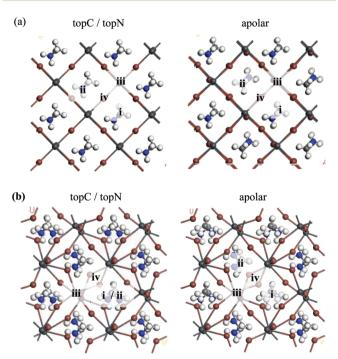
Fig. 3 Position of a fullerene  $C_{60}$  on (a) cubic and (b) tetragonal MAPbl<sub>3</sub>(001) surfaces with MAI terminations for topC/topN and apolar geometries: (i) aboveC, (ii) aboveN, (iii) abovel, and (iv) bridge. H, C, N, I, and Pb atoms are represented by the white, light grey, blue, brown, and dark grey spheres, respectively. H, C, N, I, and Pb atoms are represented by the white, light grey, blue, brown, and dark grey spheres, respectively.
