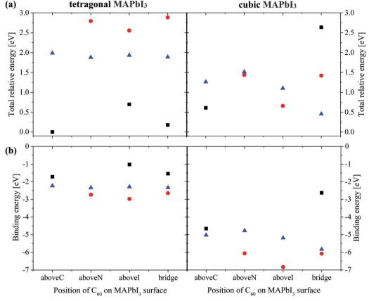
Fig. 5 (a) Total DFT-D and (b) binding energies of a MAPbl<sub>3</sub>/C<sub>60</sub> heterojunction relative to the topC-aboveC configuration. Orientations of the MA cation with respect to the (001) surface are: topC (black), topN (red) and apolar (blue).
