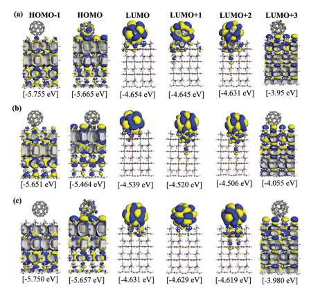
Fig. 4 Calculated Kohn-Sham orbitals and energy eigenvalues of a MAPbl $_3$ /C $_{60}$  heterojunction with tetragonal MAPbl $_3$  from HOMO-1 to LUMO+3 levels. Yellow and blue denote plus and minus regions of the orbitals. The perovskite has a topC geometry with a fullerene C $_{60}$  on the (a) aboveC, (b) abovel and (c) bridge positions.
