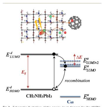
Fig. 1 Schematic illustration of the energy-level diagram for the MAPbI<sub>3</sub> and  $C_{60}$  in the hybrid perovskite/fullerene heterojunction.  $E_q$  is the energy gap of MAPbI<sub>3</sub> and  $\Delta E$  is the dissociation energy of the electron-hole pairs. The three-fold degenerate LUMO of  $C_{60}$  fullerene has three energy levels from the LUMO to LUMO+2
