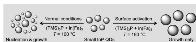
Fig. 11 (Fig. 1a in ref. 123). Two proposed reaction pathways for the growth of (\text{InP})_n quantum dots (QD) starting with the amine-based pre-synthesized seeds of InP QDs plus In(III) alkanoate, \text{In}(\text{Fa})_3 (Fa = fatty acid carboxylate anion), and tris(trimethylsilyl)phosphine, (\text{TMS})_3\text{P} , in the absence (left) or presence (right) of the surface-activation reagent acetylacetone. Reproduced with permission from ref. 123. Copyright 2017 Springer.
