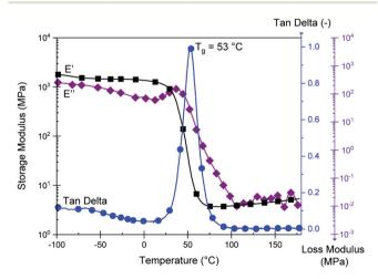
Fig. 5 DMTA data (-100 °C to 180 °C, 1 Hz, 0.1% strain) of cured CBDA-2/ELO thermosets using a fixed COOH/oxirane group-ratio of 0.8 (the symbols are intended to help differentiate the curves and do not represent the sole data points).
