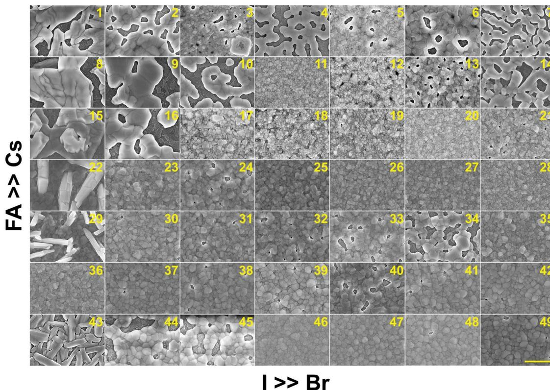
Fig. 7 Top-view SEM images of the perovskite films in the  $\text{Cs}_y\text{FA}_{1-y}\text{Pb}(\text{Br}_x\text{I}_{1-x})_3$  compositional space. The panels are arranged in the same order as in the composition matrix of Fig. 1A. The yellow scale bar on the right bottom is 1  $\mu\text{m}$ .
