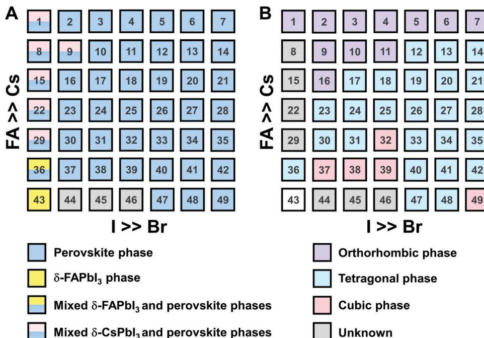
Fig. 6 Color map of the presence of perovskite phases (A) and the presence of crystal symmetry for perovskite phases (B) in the  $\text{Cs}_x\text{FA}_{1-x}\text{Pb}(\text{Br}_y\text{I}_{1-y})_3$  compositional space based on the XRD and GIWAXS data. (B) only show the crystal symmetry for the perovskite phases in (A) and the empty square for  $\text{FAPbI}_3$  (No. 43) is non-perovskite phase.
