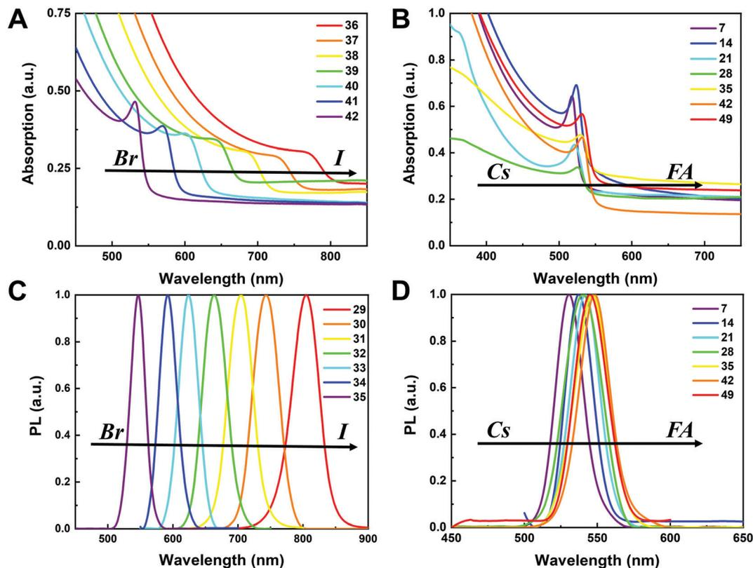
Fig. 8 Ultraviolet-visible absorbance spectra of  $\text{Cs}_{1/6}\text{FA}_{5/6}\text{Pb}(\text{Br}_x\text{I}_{1-x})_3$  (A) and  $\text{Cs}_y\text{FA}_{1-y}\text{PbBr}_3$  (B) films. Normalized photoluminescence spectra of  $\text{Cs}_{2/6}\text{FA}_{4/6}\text{Pb}(\text{Br}_x\text{I}_{1-x})_3$  (C) and  $\text{Cs}_y\text{FA}_{1-y}\text{PbBr}_3$  (D) films.
