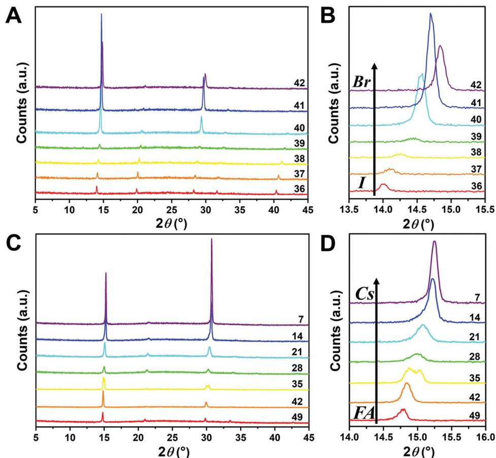
Fig. 4 XRD patterns of  $\text{Cs}_{1/6}\text{FA}_{5/6}\text{Pb}(\text{Br}_{x1-x})_3$  films as a function of the Br content (A and B) and  $\text{Cs}_\gamma\text{FA}_{1-y}\text{PbBr}_3$  as a function of the Cs content (C and D). (B) and (D) are expanded views of the peaks at  $\sim 14-15^\circ$  in (A) and (C).
