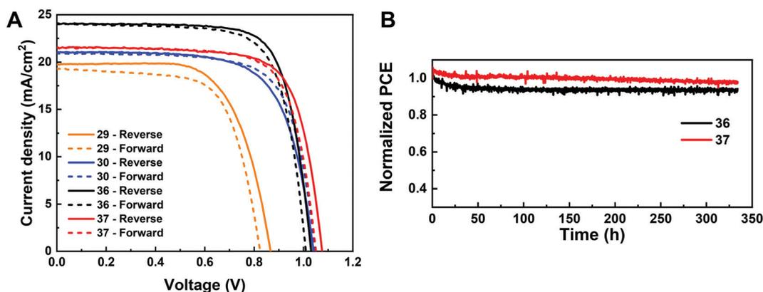
**Fig. 11** (A) Reverse  $J$ - $V$  curves of the champion PSCs of composition No. 29, 30, 36, and 37 using 1.0 M perovskite precursor solutions with 5% excess Pb<sup>2+</sup>. (B) Continuous MPP tracking results under 1 Sun irradiation in a N<sub>2</sub> atmosphere for devices of composition No. 36 and 37.
