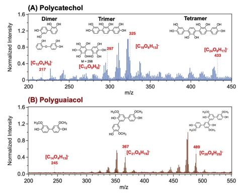
Fig. 8 Representative MALDI-TOF mass spectrum of (A) polycatechol and (B) polyguaiacol thin films in the negative ion reflector mode, [M-H]<sup>-</sup>. The structure of fragments was based on ref. 207 for polycatechol and ref. 208 for polyguaiacol. No additional matrix compound was used in the spectra collection. Spectra were collected with the assistance of Dr Lauren T. Fleming, Prof. Sergey A. Nizkorodov, and Dr Ben Katz at the University of California Irvine Mass Spectrometry Facility
