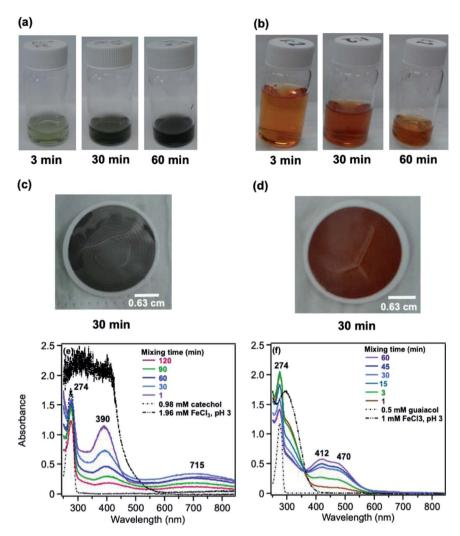
Fig. 6 Dark reaction of catechol and quaiacol with FeCl<sub>3</sub> at pH 3: (a and b) digital images of the 1: 2 organic reactant/Fe molar ratio of unfiltered solutions as a function of time; (c and d) particles on filter after 30 min; and (e and f) the corresponding UV-vis spectra after filtration. Reproduced from ref. 70 with permission from the American Chemical Society, © 2015.
