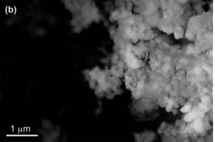
Fig. 7 SEM images of (a) polycatechol and (b) polyguaiacol collected on copper grids after a 90 min dark reaction of catechol with FeCl $_3$  at pH 3 in a 1 : 2 molar ratio. Reproduced from ref. 70 with permission from the American Chemical Society © 2015.
