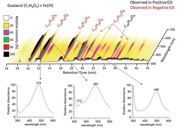
Fig. 11 (Upper panel) HPLC/PDA chromatogram of quaiacol/Fe(III) reaction products. The x-axis is the retention time, the y-axis is the UV-vis absorption wavelength, and color denotes the intensity of the absorption signal. (Lower panels) UV-visible spectra of selected chromophores. The figure and the caption were reproduced from ref. 211 with permission from the American Chemical Society, © 2017.
