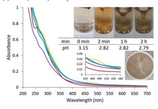
Fig. 20 UV-Vis absorption spectra of mixture of excess Fe(iii) and BBOA extracts. Different colors of traces correspond to the spectra of BBOA before mixing (red), 2 min after mixing (orange), 30 min after mixing (green), 1 h after mixing (light blue), 2 h after mixing (dark blue), and filtered solution (purple). Reproduced from ref. 190 under Create Commons License (CC BY-NC) from the Royal Society of Chemistry, © The Author(s), 2021.
