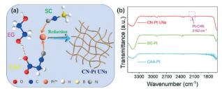
Fig. 2 (a) Schematic diagram of CN-Pt UNs; (b) FT-IR spectra of CN-Pt UNs, SC-Pt NPs and CAA-Pt NNs.
