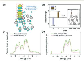
Fig. 1 (a) Differential charge density of CN-Pt UNs, where the isosurface value is 0.003 e bohr<sup>-3</sup>. The light yellow and blue regions in the diagram represent the gain and loss of electrons, respectively. (b) Bader charge population of the different elements in CN-Pt UNs. Orbital-decomposed partial density of states of (c) Pt and (d) CN-Pt UNs in the nanocontact model.
