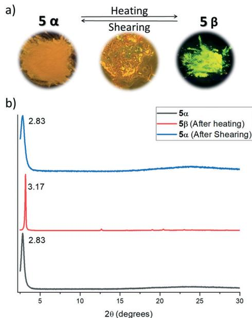
**Fig. 7** (a) Photographs of the interconversion between polymorphs  $5\alpha$  and  $5\beta$  illuminated with a 365 nm lamp. (b) Thermal and subsequent mechanochemical polymorphic transformations followed by powder X-ray diffraction pattern changes.
