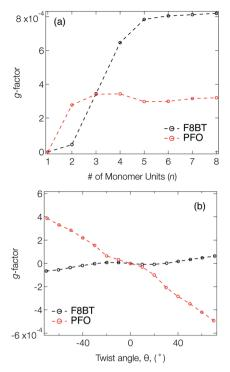
Fig. 2 (a) g-Factor of the S<sub>1</sub> state as a function of the number of monomer units (n) for PFO (red) and F8BT (black) oligomers. A fixed twist angle ( $\theta = 40^{\circ}$ ) was used throughout. (b) g-Factor as a function of  $\theta$  for PFO (red) and F8BT (black) 2-mers (n = 2). The dashed line between the points are a guide for the eye.
