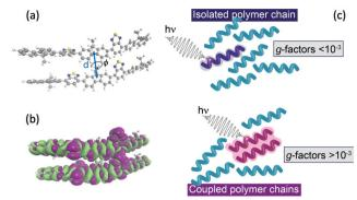
Fig. 4 (a) Schematic of two polymer chains and the coordinates (d and  $\phi$ ) manipulated in Fig. 3. (b) Density difference of the lowest exciton of a F8BT dimer model illustrating the electron density delocalised over the two chains. (c) Schematic of the effect of interacting polymer chains on the electric and magnetic transition dipole moments.
