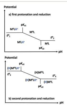
Fig. 15 Representation of the Pourbaix diagram of a given catalyst based on a CECE sequence with MLH the ligand protonated species and (H)M the hydride intermediates. The horizontal lines are plotted with respect to the reduction potentials of the catalyst, while vertical lines are plotted for its  $pK_a$  values. Diagonal lines separate processes involving a simultaneous oxidation and protonation process.
