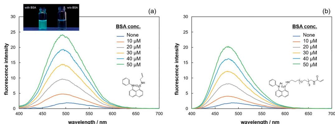
Fig. 1 Fluorescence intensity of the ANS-based monomers with different BSA concentrations. (a) ANS monomer with a photograph, (b) PEG-ANS monomer.
