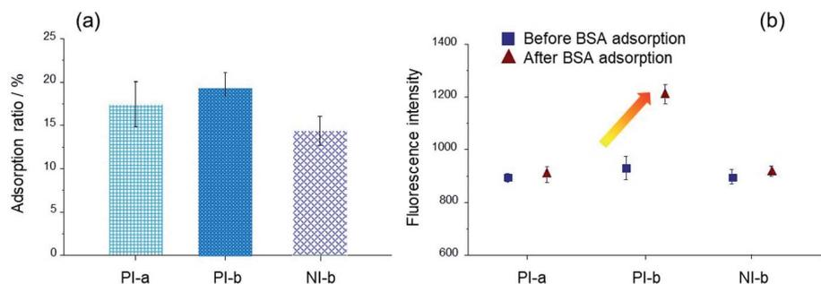
Fig. 2 Adsorption of BSA on the hydrogels. (a) Adsorption ratio of BSA for each hydrogel, (b) fluorescence intensity of each hydrogel with/without BSA.
