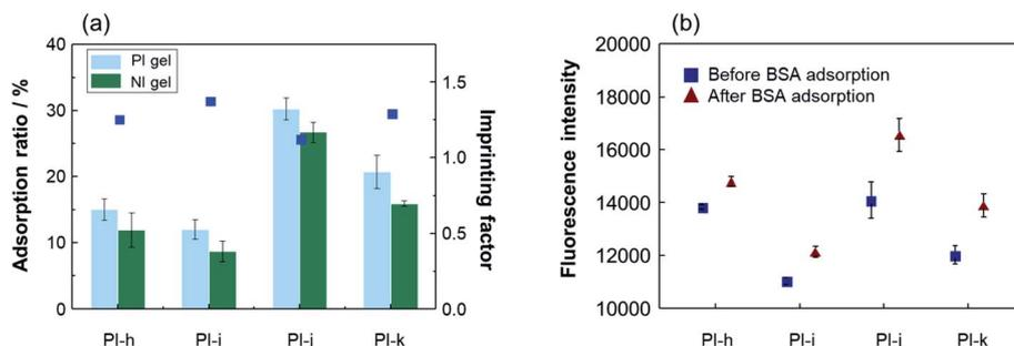
Fig. 4 Adsorption of BSA on PI gels with the PEG-ANS monomer. (a) Adsorption ratio of BSA in each hydrogel, (b) fluorescence intensity of each hydrogel with/without BSA.
