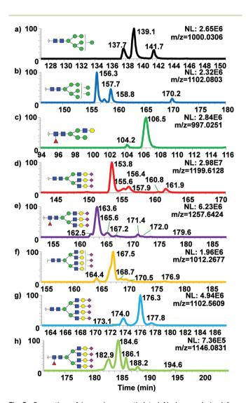
Fig. 5 Separation of isomeric permethylated N-glycans derived from human blood serum using 200 cm µPAC. EICs of various permethylated N-glycans derived from human blood serum using µPAC are shown. (a) Man7, (b) Man8, (c) GlcNAc3Man3Gal1deoxyHex1, (d) GlcNAc5Man3Hex3NeuAc3, (e) GlcNAc5Man3Hex3deoxyHex1NeuAc3, (f) GlcNAc6Man3Hex4NeuAc3, (g) GlcNAc6Man3Hex4NeuAc4 and (h) GlcNAc6Man3Hex4deoxyHex1NeuAc4.
