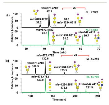
Fig. 6 Analysis of permethylated O-glycans using 50 and 200 cm  $\mu$ PAC. EIC of permethylated O-glycans derived from  $\kappa$ -casein and bovine fetuin using (a)  $\mu$ PAC 50 cm and (b)  $\mu$ PAC 200 cm. Upper panel of each figure depicts permethylated O-glycans derived from  $\kappa$ -casein and bottom panel shows permethylated O-glycans derived from bovine fetuin
