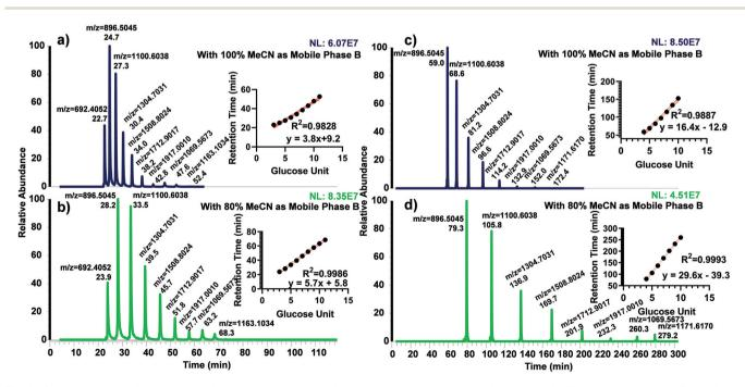
Fig. 1 Chromatograms of permethylated dextran ladder and their correlation against the retention time with different mobile phase B conditions. (a) Permethylated dextran ladder with  $\mu$ PAC 50 cm and 100% MeCN as mobile phase B. (b) Permethylated dextran ladder with  $\mu$ PAC 50 cm and 80% MeCN as mobile phase B. (c) Permethylated dextran ladder with  $\mu$ PAC 200 cm and 100% MeCN as mobile phase B. (d) Permethylated dextran ladder with  $\mu$ PAC 200 cm and 80% MeCN as mobile phase B.
