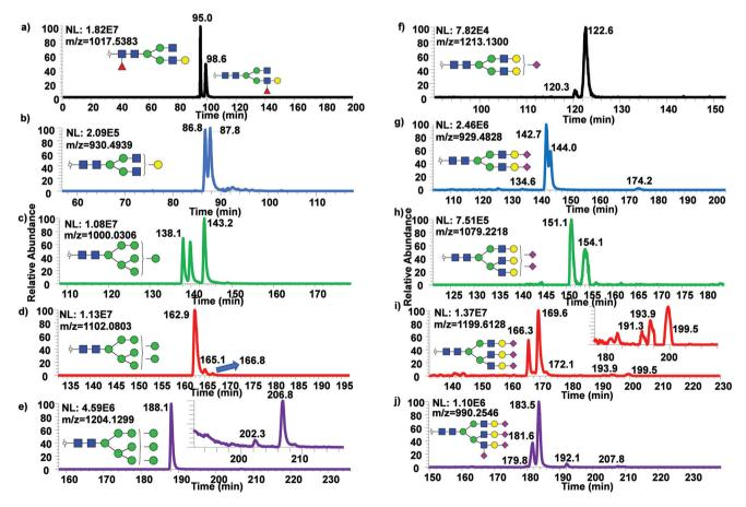
Fig. 4 Isomeric separation of permethylated two *N*-glycan standards (a) and *N*-glycans derived from model glycoproteins using 200 cm μPAC. EIC of permethylated *N*-glycans derived from mouse immunoglobin G (b), ribonuclease B (c–e) and bovine fetuin (f–j) using μPAC 200 cm column.
