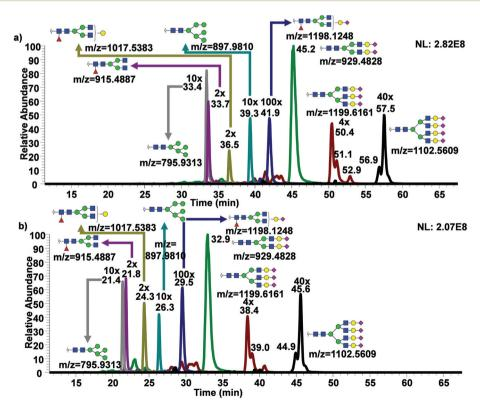
Fig. 3 Effects of higher flow rate for the permethylated glycan analysis using 50 cm µPAC. EIC of permethylated N-glycans derived from human blood serum using µPAC 50 cm at (a) 300 nL min<sup>-1</sup> flow rate and (b) 600 nL min<sup>-1</sup>. There are noticeable changes in retention time due to the increase in flow rate. Zoom factors such as " $10\times$ " indicate zoom in y-axis.
