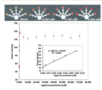
Fig. 3 Visual calibration curve was generated for semi-quantitative Hg (II) determination (top). Hg(II) calibration curve was produced in the range of 0.001–0.060 mM by analyzing the green intensity of the color change in the detection zone (bottom).
