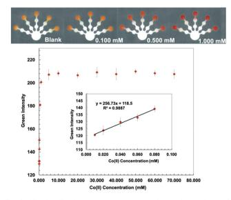
Fig. 4 Visual calibration curve was generated for semi-quantitative Co (II) determination (top). Co(II) calibration curve was produced in the range of 0.010-0.080 mM by analyzing the green intensity of the color change in the detection zone (bottom).
