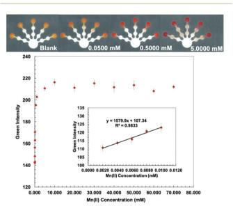
Fig. 5 Visual calibration curve was generated for semi-quantitative Mn (II) determination (top). Mn(II) calibration curve was produced in the range of 0.0020-0.0100 mM by analyzing the green intensity of the color change in the detection zone (bottom).
