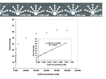
Fig. 2 Visual calibration curve was generated for semi-quantitative Cu(III) determination (top). Cu(III) calibration curve was produced in the range of 0.005–1.000 mM by analyzing the gray intensity of the color change in the detection zone (bottom).
