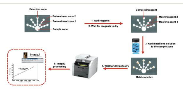
Fig. 1 The process of fabricating  $\mu PAD$  and detecting Cu(ii), Co(ii), Ni(ii), Hg(ii), and Mn(ii).
