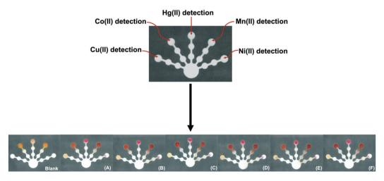
Fig. 7 The color change of the metal complexes for simultaneous detection of the five metal ions on one device of (A) 1:1 ratio for all five metal ions, (B) 1:2 for Cu(n): other metal ions, (C) 1:2 for Cu(n): other metal ions, (E) 1:2 for Cu(n): other metal ions.
