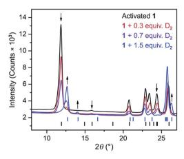
Fig. 4 Rietveld refinement fits of powder neutron diffraction patterns ( $\lambda=2.0772$  Å, T=9 K) collected for activated 1 and activated 1 dosed with 0.3, 0.7, and 1.5 equiv. of D<sub>2</sub> per pore. Black (lower) and blue (upper) tick marks indicate calculated Bragg peak positions for 1 and the D<sub>2</sub> adsorbed phase,  $1-D_2$ , respectively. Arrows indicate peaks that best illustrate the conversion of 1 to  $1-D_2$  with increasing D<sub>2</sub> loading.
