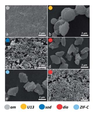
Fig. 4 SEM micrographs of the biocomposites am (a) and U13 (b, from TD-H<sub>2</sub>O), sod (c, from TD-EtOH), dia (from TD-H<sub>2</sub>O) do and from TD-EtOH (f)) and ZIF-C (e, from TD-H<sub>2</sub>O) phases. ZIF-C refers to  $ZIF-CO_{3-140}$
