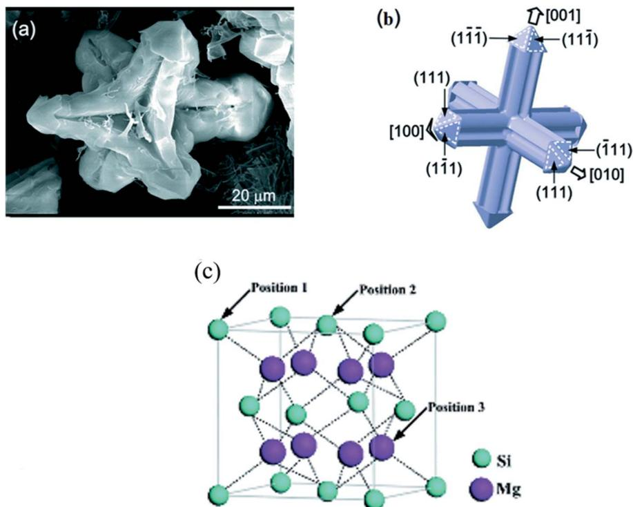
Fig. 3 (a and b) Structure and planes of the primary  $Mg_2Si$  phase. (c) Molecular structure of the  $Mg_2Si$  phase. This figure has been reproduced from ref. 23 with permission from Royal Society of Chemistry, copyright 2014.
