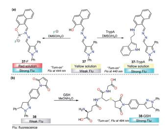
Fig. 17 Probes for tryptamine based on pyrazoles (a) 37 and (b) 38.
