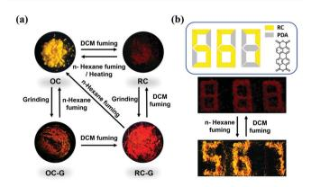
Fig. 7 (a) FL images of the crystal-to-crystal switching processes in response to multiple stimuli. (b) Application of the RC responsive behavior to solvent vapor in FL encryption: a pattern "888" is drawn with RC (yellow) and 3,4,9,10-perylenetetracarboxylic dianhydride (PDA) (gray). The red pattern is reversibly switched to orange pattern "567" upon vapor fuming.
