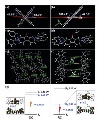
Fig. 3 Dihedral angle of DCzFO in (a) OC and (b) RC crystals. Twisted molecular conformation of DCzFO in (c) OC and (d) RC crystals. (e) Intermolecular interactions between adjacent molecules of the OC crystal. (f) Two adjacent dimers and intermolecular interactions of DCzFO and DCM in the RC crystal. (g) Theoretically calculated vertical excitation energies, transition natures of the excited states and oscillator strengths (f) for OC and RC. Interaction distances (dashed lines) are in Å.
