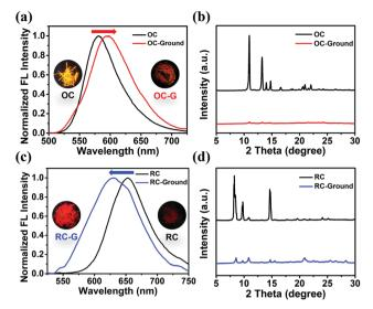
Fig. 6 (a) Normalized FL spectra ( $\lambda_{ex}$  = 400 nm) and (b) PXRD patterns of **OC** before and after being ground. (c) Normalized FL spectra ( $\lambda_{ex}$ 400 nm) and (d) PXRD patterns of RC before and after being ground.
