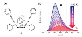
Fig. 11 (a) Molecular structure of Au(ı) complex 12. (b) Temperaturedependent emission spectral changes of 12 in the range of 180-298 K ( $\lambda_{\rm ex}$  = 340 nm). Reprinted with permission from ref. 100. Copyright 2019 American Chemical Society.
