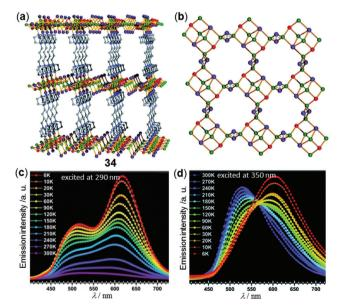
Fig. 28 (a) Independent 3D framework pillared-layered structure and (b) copper-halide single layer structure of Cu-MOF 34. (c and d) Temperature-dependent solid-state emission spectral changes of 34 in the range of 6-300 K excited at (c) 290 nm or (d) 350 nm. Reprinted with permission from ref. 65. Copyright 2018 The Royal Society of Chemistry.
