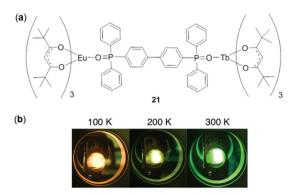
Fig. 19 (a) Molecular structure of the Eu/Tb hetero-dimetallic complex 21. (b) Photographs showing emission colors of 21 at 100, 200, and 300 K, respectively. Reprinted with permission from ref. 113. Copyright 2018 Wiley-VCH.
