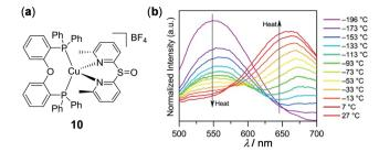
Fig. 9 (a) Molecular structure of Cu(ı) complex 10. (b) Normalized temperature-dependent emission spectral changes of 10 from -196 to 27 °C as thin films by drop-casting on quartz from MeOH solution ( $\lambda_{ex}$  = 380 nm). Reprinted with permission from ref. 99. Copyright 2018 American Chemical Society.
