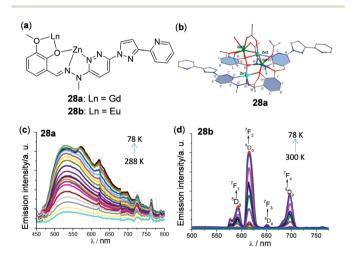
Fig. 24 (a) Structure segment of the Zn<sub>2</sub>Ln<sub>2</sub> clusters 28a and 28b. (b) Cation core structure of 28a. (c and d) Temperature-dependent emission spectra of (c) 28a (78-288 K) and (d) 28b (78-300 K) with excitation at 350 nm. The three sharp peaks marked with a gray rectangle in panel (c) are the emission spectra of a background light source. Reprinted with permission from ref. 125. Copyright 2017 American Chemical Society.
