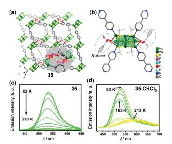
Fig. 29 (a) Two-layer stack and (b) perspective view of the coordination environment of Aq-MOF 35. (c and d) Temperature-dependent solidstate emission spectral change of (c) 35 and (d) 35·CHCl<sub>3</sub>. Reprinted with permission from ref. 131. Copyright 2018 American Chemical Society
