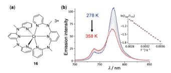
Fig. 15 (a) Molecular structure of Cr(III) complex 16 with BF<sub>4</sub> counter anions. (b) Temperature-dependent emission spectra of 16 in air-saturated H<sub>2</sub>O from 278 to 358 K. Inset: The related Boltzmann fitting plots of  $ln(I_{738}/I_{775})$  vs.  $T^{-1}$ . The emission changes are reversible. Reprinted with permission from ref. 104. Copyright 2017 Wiley-VCH.
