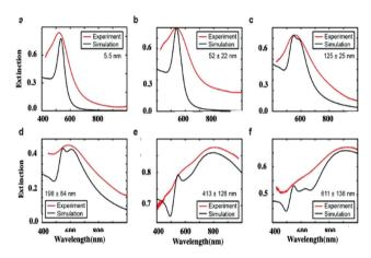
Fig. 10 Extinction spectra of isolated Au nanocrystals and assemblies of various sizes. (a)  $5.5 \pm 0.4$  nm Au nanocrystals; Au aggregates with sizes of (b) 52  $\pm$  22 nm, (c) 125  $\pm$  25 nm, and (d) 198  $\pm$  84 nm; Au supracrystals with sizes of (e) 413  $\pm$  128 nm and (f) 611  $\pm$  138 nm. The average sizes were used to fit the measured data.
