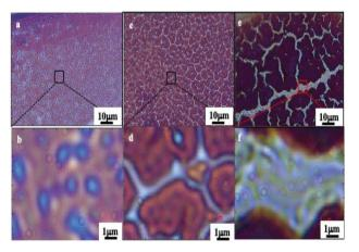
Fig. 4 Optical micrographs of the 0.2-0.6 µm supracrystal film, in the transmission mode. (a and b), 0.4-1.0 µm (c and d) and 1.0-1.4 µm (e and f).
