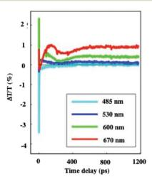
Fig. 12 Dynamics of the  $\Delta T/T$  at selected probe wavelengths, on nanometer time scales of energy flow in the Au clustered structures.
