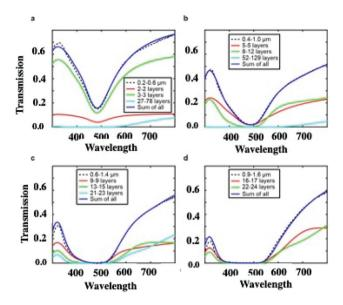
Fig. 8 Calculated (blue solid traces) and experimental (dashed traces) transmission spectra of 8.2 nm Ag NC supracrystal films with various thicknesses. (a)  $0.2-0.6~\mu m$ , (b)  $0.4-1~\mu m$ , (c)  $0.6-1.4~\mu m$ , and (d) 0.9-1.6 µm. The calculated spectra account for wetting layers with different thicknesses. Colors correspond to different numbers of monolayers.
