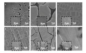
Fig. 3 SEM images of supracrystal films of 8.2 nm Ag nanocrystals with various thicknesses. (a)  $0.2-0.6~\mu m$ , (b)  $0.4-1.0~\mu m$ , (c)  $0.6-1.4~\mu m$ , (d)  $0.9-1.6 \mu m$ , (e)  $1-1.4 \mu m$  and (f)  $1.3-1.9 \mu m$ .
