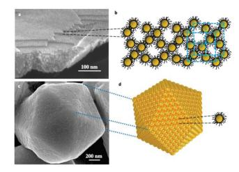
Fig. 1 Supracrystals grown under heterogeneous (a and b) and homogeneous (c and d) conditions. SEM images of nanocrystals self-assembled layer by layer (a) and shaped supracrystals (b) of 5 nm Au nanocrystals coated with dodecanthiol. Scheme of such fcc supracrystals (b and d).
