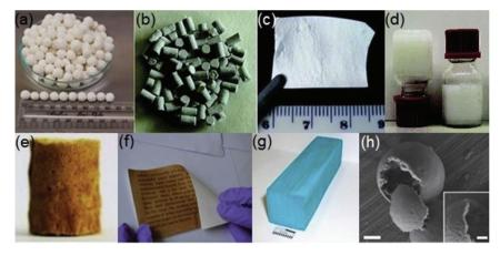
Fig. 1 Examples showing different shapes of MOFs: (a) granule, (b) pellet, (c) thin film, (d) gel, (e) foam, (f) paper sheet, (g) monolith and (h) hollow structure (scale bar 500 nm (inset 200 nm)). Reprinted with permission from ref. 83. Copyright 2018 Elsevier.
