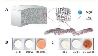
Fig. 8 (A) The schematic representation of a MOF-cellulose hybrid aerogel. Photographs of (B) CNC-CMC-MOF based hybrid aerogels (CNC:CMC:MOF = 1:1:1) by weight), and (C) all-CNC-MOF based hybrid aerogels (CNC: CNC: MOF = 1:1:1 by weight); aerogels are about 7 mm in diameter and 5 mm in height. Reprinted with permission from ref. 123. Copyright 2016 John Wiley and Sons.
