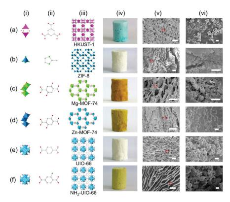
Fig. 10 The crystal structures of HKUST-1, ZIF-8, Mg-MOF-74, Zn-MOF-74, UIO-66, and NH<sub>2</sub>-UiO-66, and the optical photos and SEM images of the MOF@CMC foams based on these MOFs. The scale bars are 100 µm in v and 1 µm in vi. Reprinted with permission from ref. 133. Copyright 2016 American Chemical Society.
