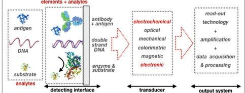
the components of a biosensor
