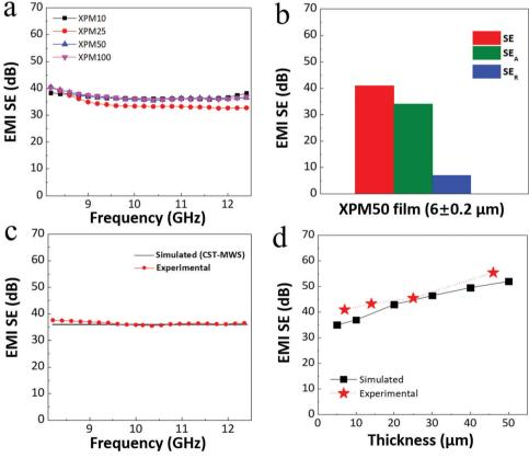
Fig. 5 (a) Recorded EMI SE of different crosslinked PEDOT:PSS-Ti<sub>3</sub>C<sub>2</sub>T<sub>x</sub> MXene nanocomposite films, viz. XPM10, XPM25, XPM50 and XPM100 in the X-band (8.2–12.4 GHz). (b) Recorded average EMI SE<sub>A</sub> and SE<sub>R</sub> values of the XPM50 film for a thickness of 6  $\pm$  0.2  $\mu$ m. (c) Comparison of the CST-MWS simulated and experimental EMI SE of the XPM50 film. (d) Thickness dependent average EMI SE of the XPM50 film
