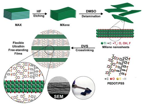
Fig. 1 Schematic of the preparation process of the crosslinked PEDOT: PSS-Ti<sub>3</sub>C<sub>2</sub>T<sub>x</sub> MXene nanocomposite film (the insets show an SEM cross-section image and a photograph of the flexible nanocomposite film).
