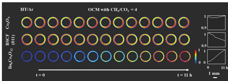
Fig. 2 Distribution of membrane components during the high temperature XRD-CT scan and OCM reaction. Plots on the right correspond to changes in the normalised scale factors of  $\text{Co}_3\text{O}_4$  and  $\text{Ba}_6\text{Co}_4\text{O}_{12}$  and the peak intensity of the BSCF (011) reflection.
