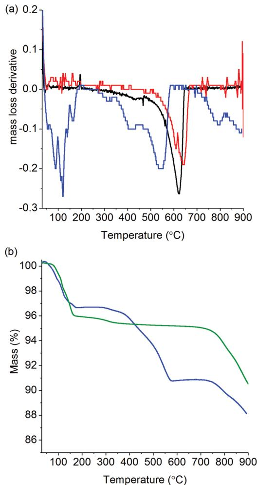
Fig. 1 Thermogravimetric analysis of soot oxidation. Experiments performed under an air atmosphere with a ramp rate of 5 °C min<sup>-1</sup>. (a) Derivative of mass losses of soot (black line), α-Al<sub>2</sub>O<sub>3</sub> + soot (red line) and K/α-Al<sub>2</sub>O<sub>3</sub> + soot (blue line). (b) Thermogravimetric profile of K/α-Al<sub>2</sub>O<sub>3</sub> + soot decomposition (blue line) and K/α-Al<sub>2</sub>O<sub>3</sub> (green line).
