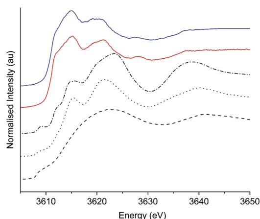
Fig. 7 Comparison of simulated potassium edge XANES of  $KHCO_3$  at different cluster sizes with experimental  $KHCO_3$  and  $K/\alpha-Al_2O_3$ . Black lines: 6 atoms (dashed), 22 atoms (dotted), 50 atoms (dashed–dotted) Red line: experimental  $KHCO_3$  and blue line  $K/\alpha-Al_2O_3$ .
