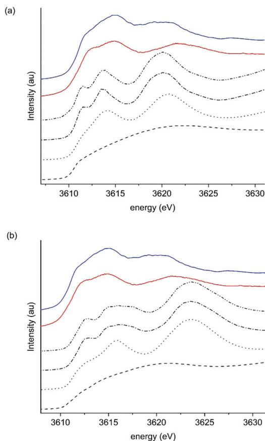
Fig. 8 Comparison of simulated potassium edge XANES of  $K_2CO_3$  at different cluster sizes with 5% expansion/contraction of the lattice. (a) 5% lattice expansion. (b) 5% lattice contraction. Black lines: 6 atoms (dashed), 22 atoms (dotted), 50 atoms (dashed–dotted). Red line: experimental  $K_2CO_3$  and blue line  $K/\alpha-Al_2O_3$ .
