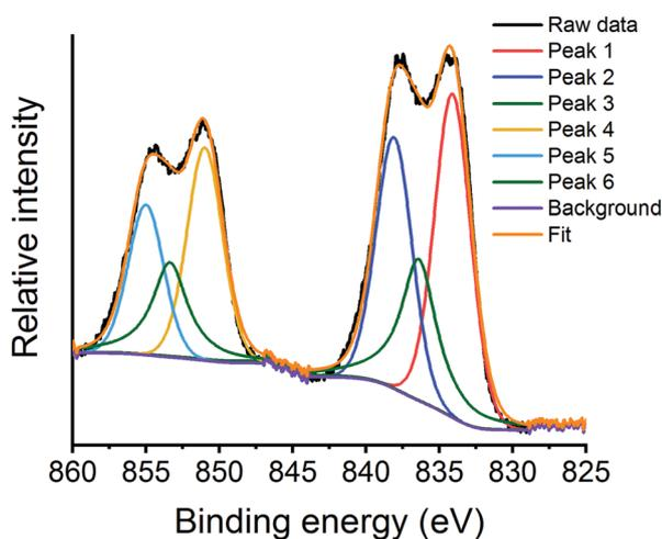
Fig. 12 La 3d XPS region for the argon milled catalyst showing the deconvoluted peaks at RT under a N<sub>2</sub>O atmosphere.
