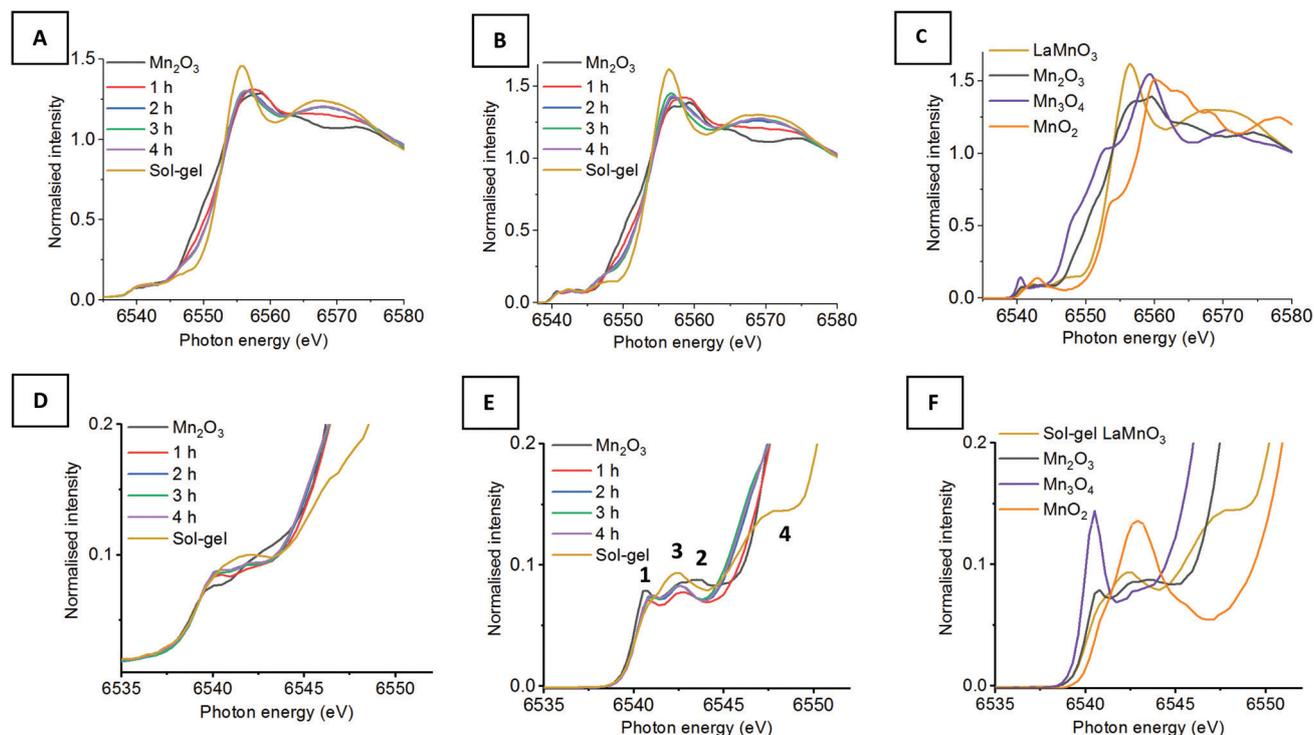
Fig. 1 (A) XAS Mn K-edge XANES compared to (B) HERFD-XANES of time-slices during the mechanochemical synthesis of LaMnO<sub>3</sub> compared to (C) reference Mn(II), (III), (IV) oxides and sol-gel synthesised LaMnO<sub>3</sub> with (D–F) their respective highlighted pre-edge region.
