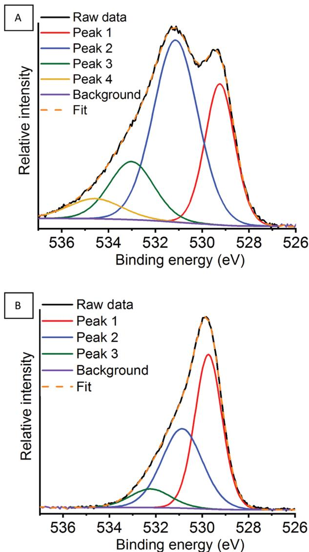
Fig. 13 O 1s region for the argon milled catalyst showing the deconvoluted peaks at (A) RT and (B) 600 °C under a N<sub>2</sub>O atmosphere.
