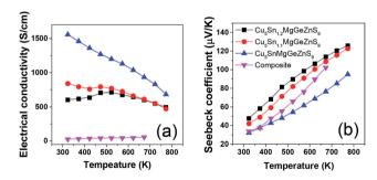
Fig. 9 Temperature dependent (a) electrical conductivity and (b) Seebeck coefficient of high entropy sulfide  $Cu_5Sn_{1+x}MgGeZnS_9$  (x = 0, 0.1, 0.2). The values for  $Cu_3SnS_4-Cu_2MgGeS_4-ZnS$  composite are also shown for comparison. Reproduced under the terms of the CC-BY 4.0 license. Copyright 2018, the authors, published by ACS Publications.<sup>7</sup>
