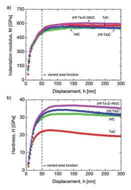
Fig. 11 Comparison of: (a) indentation modulus; and (b) hardness depth-profiles of the mono, binary and high-entropy carbide (Hf-Ta–Zr-Nb)C. The results were averaged from 64 indents made per sample, following rejection of those close to grain boundaries and pores. Reproduced under the terms of the CC-BY 4.0 license. Copyright 2018, the authors, published by Springer Nature.<sup>42</sup>
