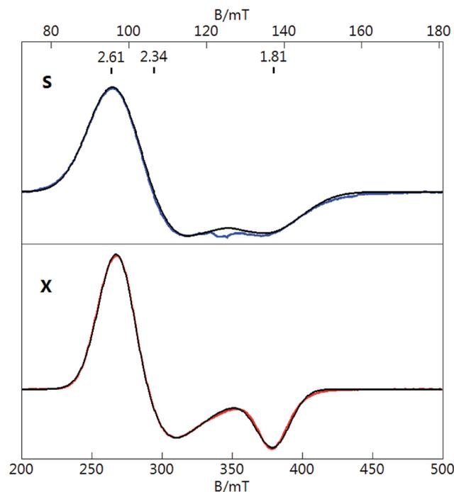
Fig. 2 S-band (3.489 GHz) and X-band (9.644 GHz) EPR spectra of  $[\text{Au}_{25}(\text{SR})_{18}]^0$  in 1 : 1  $\text{CH}_2\text{Cl}_2$  : toluene at  $T = 10$  K (S), 6 K (X). Microwave power: 0.3 mW (S), 2 mW (X). See text for parameters of simulations (black lines).
