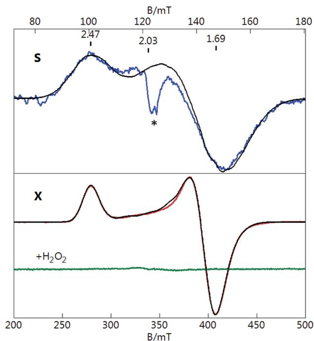
Fig. 1 S-band (3.480 GHz) and X-band (9.645 GHz) EPR spectra of  $[\text{Au}_{133}(\text{TBBT})_{52}]^0$  in 1 : 1  $\text{CH}_2\text{Cl}_2$  : toluene at  $T = 10$  K (S-band), 6 K (X-band). Microwave power: 0.3 mW (S-band), 2 mW (X-band), see text for parameters of simulations (black lines). The green trace shows loss of signal after  $\text{H}_2\text{O}_2$  addition. The  $g = 2.03$  signal (indicated by \*) is from the extraneous copper impurity.
