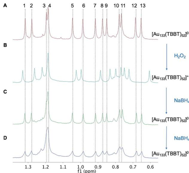
Fig. 5 Redox property of  $\text{Au}_{133}(\text{TBBT})_{52}$  probed by NMR. (A) NMR of *tert*-butyl-H in  $[\text{Au}_{133}(\text{TBBT})_{52}]^0$ . (B) Oxidation of  $[\text{Au}_{133}(\text{TBBT})_{52}]^0$  to  $[\text{Au}_{133}(\text{TBBT})_{52}]^+$  by  $\text{H}_2\text{O}_2$ . (C) Reduction of  $[\text{Au}_{133}(\text{TBBT})_{52}]^+$  to  $[\text{Au}_{133}(\text{TBBT})_{52}]^0$  by  $\text{NaBH}_4$ . (D) Further reaction of  $[\text{Au}_{133}(\text{TBBT})_{52}]^0$  with  $\text{NaBH}_4$ .
