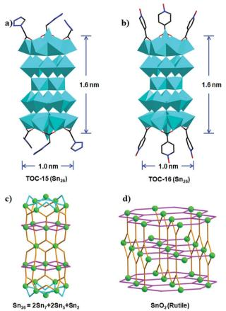
Fig. 2 Polyhedral representations of the  $Sn_{26}$  cluster in TOC-15 (a) and TOC-16 (b). The ball-and-stick representations of  $Sn_{26}$  (c) and  $SnO_2$  (rutile) (d). Polyhedral color code: blue  $SnO_5C/SnO_3C/SnO_6$ . Atom color code: green Sn.
