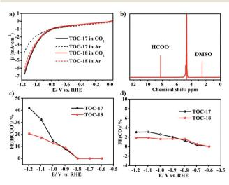
Fig. 4 (a) Linear sweep voltammetry (LSV) of TOC-17 and TOC-18 in Ar or CO $_2$  saturated 0.5 M KHCO $_3$  solution. (b)  $^1$ H NMR spectrum of the KHCO $_3$  catholyte after 3600 s of CO $_2$  reduction on the TOC-17 derived electrode, E(RHE) = -1.096 V. (c) and (d) The faradaic efficiencies (FE) of formate and CO for TOC-17 and TOC-18 derived electrodes at various potentials.
