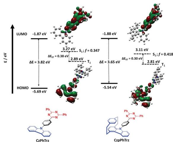
Fig. 3 DFT [PBE0/6-31G(d,p)] calculated ground and TDA-based excited state energies and electron density distributions of the HOMOs and LUMOs of **CzPhTrz** (left) and **CzpPhTrz** (right),  $f$  is the oscillator strength.
