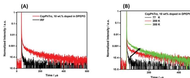
Fig. 5 (A) Time-resolved PL decay curve and (B) temperature dependence of time-resolved PL lifetime of CzpPhTrz in 10 wt% DPEPO film ( $\lambda_{\text{exc}} = 378$  nm), IRF = instrument response function.
