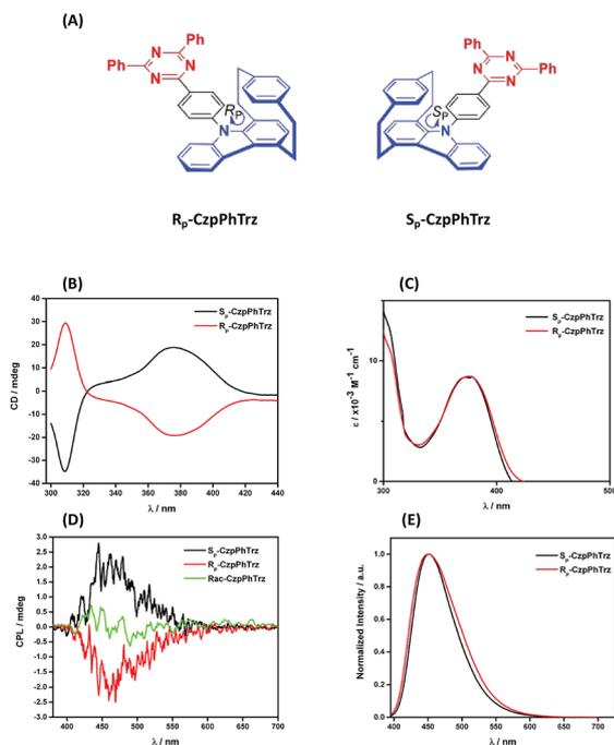
Fig. 7 (A) Chemical structures (B) CD (C) UV-vis (D) CPL and (E) PL spectra of (*R<sub>p</sub>*)-**CzpPhTrz** and (*S<sub>p</sub>*)-**CzpPhTrz** in degassed PhMe ( $\lambda_{\text{exc}} = 375$  nm).
