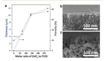
Fig. 6 Phenolic membranes prepared at different molar ratios of  $ZnCl_2$  to P123. (a) Thickness and porosity; (b, c) the cross-sectional SEM images detailing the morphology near the top surface of the membrane prepared at the molar ratios of (b) 70 and (c) 280.
