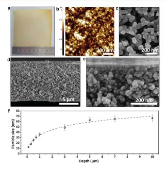
Fig. 1 Phenolic membranes with a gradient nanoporous structure. (a) The photograph of the membrane; (b) the AFM topography image of the top surface; (c) the SEM image of the bottom surface; (d) the SEM image of the cross section and (e) the enlarged image of the boxed area in (d); (f) the size of phenolic particles at different depths across the membrane.
