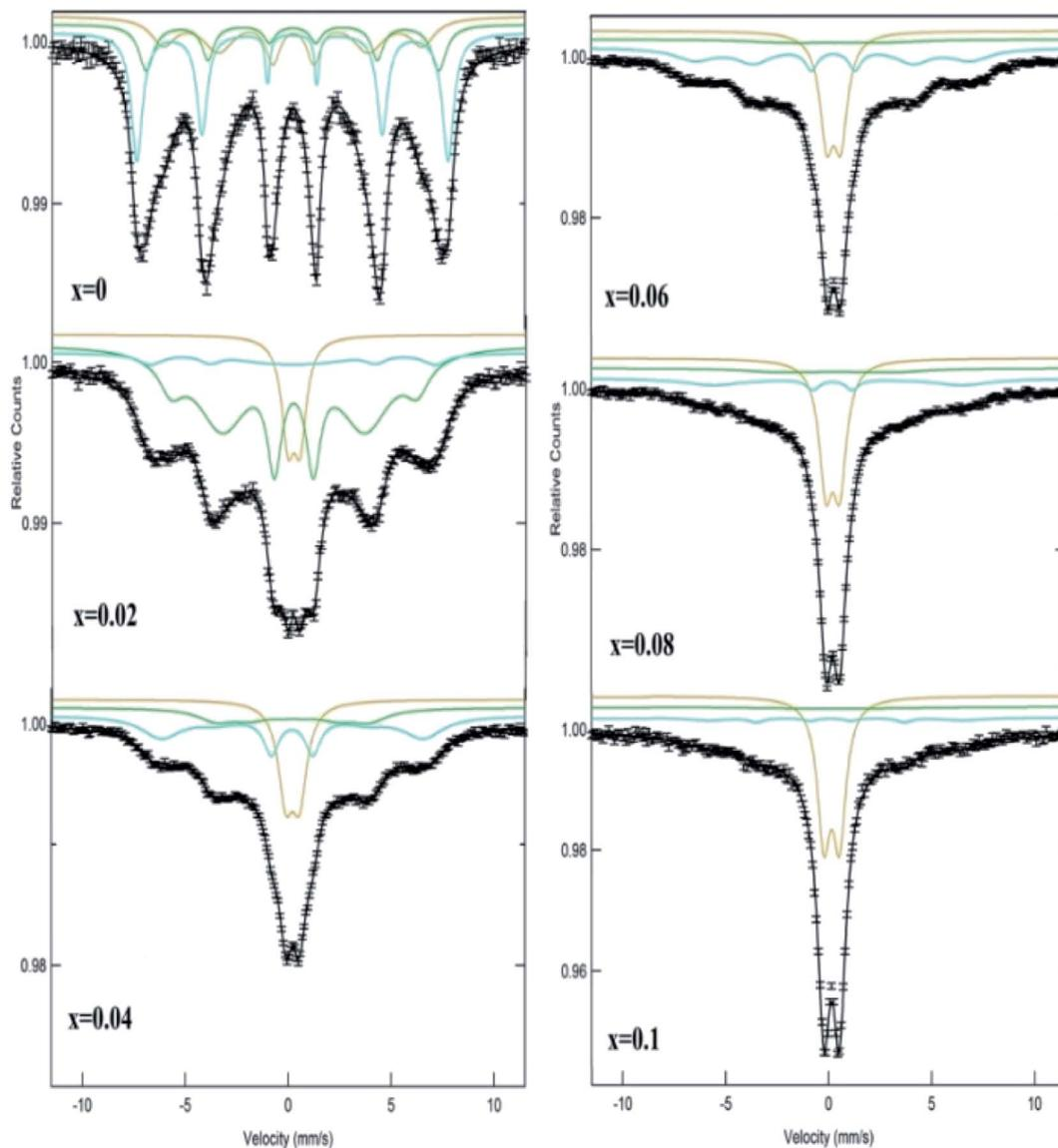
Fig. 7 RT Mössbauer spectra of  $\text{Ni}_{0.4}\text{Cu}_{0.2}\text{Zn}_{0.4}\text{La}_x\text{Y}_x\text{Fe}_{2-x}\text{O}_4$  ( $x = 0.00 - 0.10$ ) NSFs.
