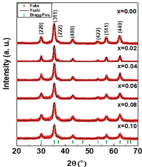
Fig. 1 XRD powder patterns of  $\text{Ni}_{0.4}\text{Cu}_{0.2}\text{Zn}_{0.4}\text{La}_x\text{Y}_x\text{Fe}_{2-x}\text{O}_4$  ( $x = 0.00 - 0.10$ ) NSFs.
