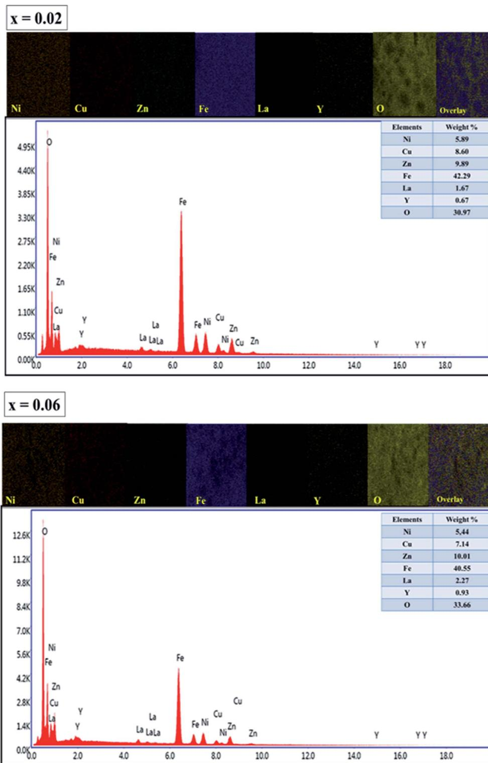
Fig. 3 EDX spectra and elemental mapping of  $\text{Ni}_{0.4}\text{Cu}_{0.2}\text{Zn}_{0.4}\text{La}_x\text{Y}_x\text{Fe}_{2-x}\text{O}_4$  ( $x = 0.00 - 0.10$ ) NSF's for  $x = 0.02$  and  $0.06$  compositions.
