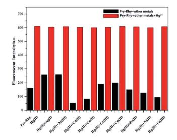
Fig. 7 The black bars represent the fluorescent intensity of sensor Pyr-Rhy and various metal ions (1.0 equiv.) in DMSO/ $H_2O$  (1/1, v/v) solution; the red bars represent the fluorescent intensity of sensor Pyr-Rhy and  $Hg^{2+}$  (1.0 equiv.) in DMSO/ $H_2O$  (1/1, v/v) solution.
