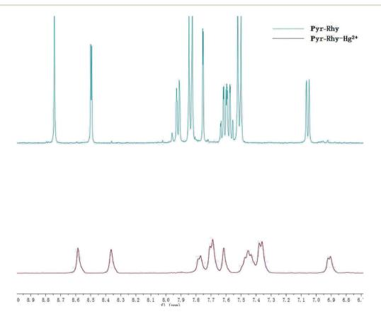
Fig. 11 <sup>1</sup>H NMR spectra of sensor Pyr-Rhy and complex Pyr-Rhy-Hg<sup>2+</sup> in DMSO-d<sub>6</sub>.
