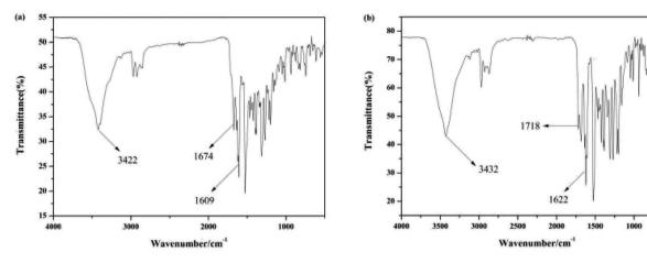
Fig. 10 (a) The FT-IR spectrum of sensor Pyr-Rhy; (b) binding FT-IR spectrum of Pyr-Rhy-Hg<sup>2+</sup>.
