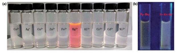
Fig. 4 (a) Colorimetric performance of sensor Pyr-Rhy (10  $\mu$ M) upon addition of different metal ions (1.0 equiv.) in DMSO/H<sub>2</sub>O (1/1, v/v) solution; (b) color change induced upon addition of Hq<sup>2+</sup> under 365 nm UV lamp.
