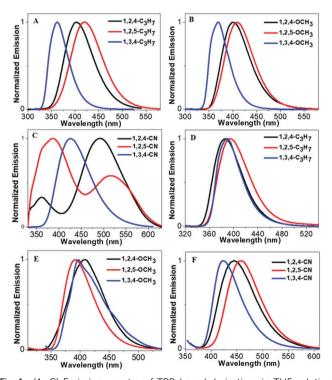
Fig. 1 (A-C) Emission spectra of TPP-based derivatives in THF solution (concentrations: 10<sup>-5</sup> M), and (D-F) emission spectra of TPP-based derivatives in the solid state.
