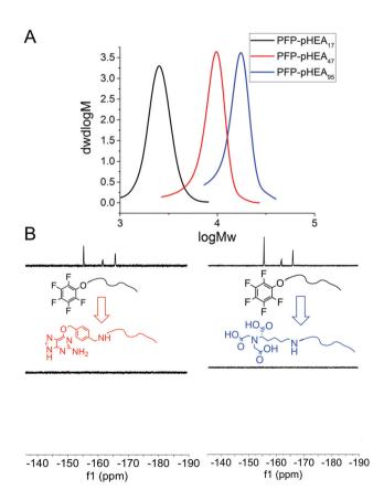
Fig. 2 (A) SEC analysis of PFP-pHEAs; (B)  $^{19}\mathrm{F-NMR}$  analysis of end group displacement.
