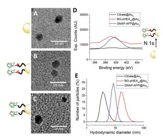
**Fig. 3** Nanoparticle characterization. (A–C) Transmission electron micrographs of citrate@Au $_4$ , SNAP-AFP-BG-pHEA $_4$ 5@Au $_4$  and His-AFP-Ni-NTA-pHEA $_{17}$ @Au $_4$  respectively; (D) N 1s peak from XPS upon conjugation of SNAP-AFP; (E) diameter from dynamic light scattering.
