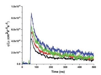
Fig. 5 Representative fp-TRMC transients with increasing fluence  $(1 \times 10^{14} - 4 \times 10^{15} \text{ photons per cm}^2)$  for a ZnPor-COF-PS film at 700 nm photoexcitation with 7 ns pulse width.
