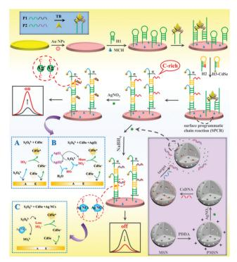
Scheme 1 Schematic diagram of the "on-off" ECL biosensing platform for versatile detection of thrombin and miRNA-21 based on Aq(ı) ionaccelerated and Ag NC-quenched ECL combined with molecular machine-triggered chain reaction and MSN double amplification.
