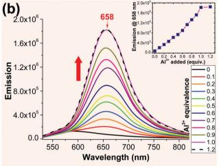
Fig. 2 Absorption (a) and emission (b) spectra recorded for probe 2 (1  $\times$  10 $^{-5}$  M) in acetonitrile upon spectrometric titration with Al $^{3+}$  (1 mM in water) at room temperature. The **2-Al** complex was excited at 507 nm to obtain the emission spectra.
