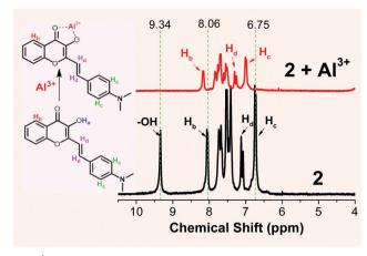
Fig. 3  $^{1}$ H NMR spectra of probe **2** in the absence (bottom) and presence (top) of one equiv. of Al $^{3+}$  (prepared from Al(NO $_3$ ) $_3\cdot$ 9H $_2$ O dissolved in acetonitrile- $d_3$ ) in deuterated DMSO- $d_6$ .
