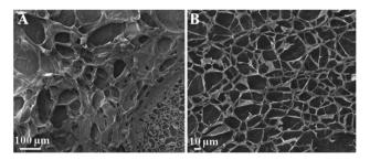
Fig. 2 SEM images of freeze-dried DNA-hydrogels with different magnifica-
