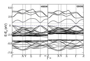
Fig. 7 Band structure for  $\text{Cu}_3\text{SbS}_4$  for spin-orbit coupling calculation with hybrid-DFT (HSE06, left panel) and QSGW (right panel). All the energies in eV referred to the Fermi energy.
