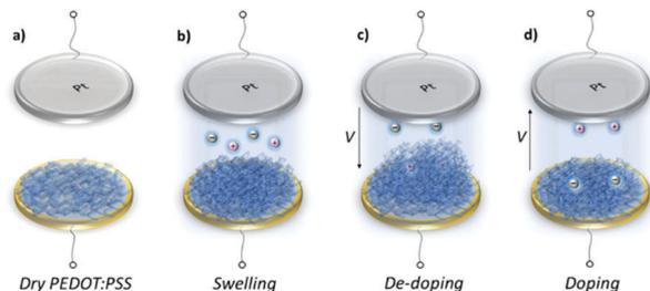
**Fig. 2** Voltage induced swelling/shrinkage of PEDOT:PSS film. (a) Dry film on a gold coated EQCM-D sensor, (b) swelling when in contact with the electrolyte, (c) additional swelling during de-doping due to up-take of  $\text{Na}^+$  ions and water, (d) shrinkage when the potential is reversed. We record significant differences in the volumetric expansion as well as the reversibility of the de-doping process depending on the film thickness.
