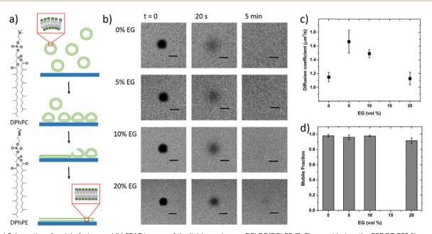
Fig. 1 (a) Schematics of vesicle fusion, and (b) FRAP images of the lipid membranes DPhPC/DPhPE (7:3) assembled on the PEDOT:PSS films cast from dispersions containing various EG concentrations (0 vol%, 5 vol%, 10 vol% and 20 vol%). These images are treated to extract diffusion coefficients (c), and mobile fractions (d) of the membrane lipids; scale bar =  $20 \mu m$ .
