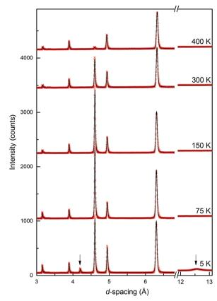
Fig. 2 Temperature evolution of the neutron diffraction pattern of MnFe<sub>3</sub>O<sub>5</sub>. Magnetic contributions appear at 300 K, and arrows indicate additional magnetic peaks at 5 K, with hkl = (001) and (003) at d-spacing = 12.6 and 4.2 Å, respectively
