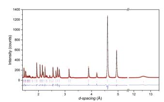
Fig. 3 Rietveld refinement of high resolution neutron diffraction patterns of MnFe<sub>3</sub>O<sub>5</sub> obtained at 5 K, with upper tick marks indicating nuclear peaks and lower presenting magnetic reflections. ( $R_{\rm wp}$  = 12.9% and  $R_{\rm p}$  = 12.6%).
