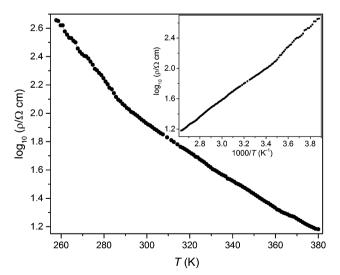
Fig. 6 Log of electrical resistivity of MnFe<sub>3</sub>O<sub>5</sub> measured between 260 and 380 K, with insert showing the plot against reciprocal temperature
