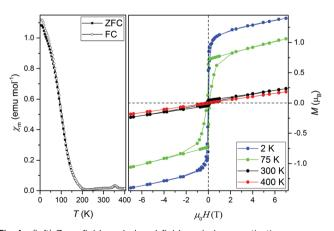
Fig. 1 (left) Zero-field cooled and field cooled magnetisation measurements between 2 and 400 K. (right) Magnetisation-field hysteresis loops for MnFe<sub>3</sub>O<sub>5</sub> measured at 2, 75, 300 and 400 K.
