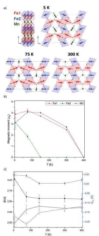
Fig. 4 (a) Magnetic structures of MnFe $_3$ O $_5$  at 5, 75 and 300 K. The network of FeO<sub>6</sub> octahedra is shown, with Mn<sup>2+</sup> in trigonal prismatic sites within channels parallel to the a-axis. (b) The temperature evolution of the ordered Mn, Fe1 and Fe2 magnetic moments. (c) Temperature evolution of BVS and  $Q_{\rm JT}$ , with closed/open symbols representing Fe1/Fe2 sites.
