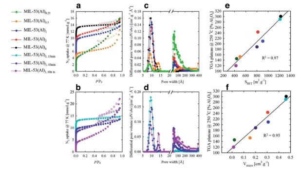
Fig. 4  $N_2$  isotherms (77 K) and pore size distributions for MIL-53(Al) materials with adjusted modulator stoichiometry/concentration (a and c) and varied reaction time (b and d); linear fits obtained by plotting (e) the BET surface areas ( $S_{BET}$ ) and (f) micro pore volume ( $V_{micro}$ ) of all 8 samples against their respective TGA plateau at 250 °C.
